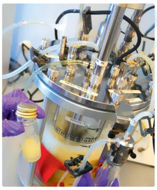
Figure 1: 5 L Electrolab Biotech Ltd bioreactor used for scale-up and scale-down studies.
