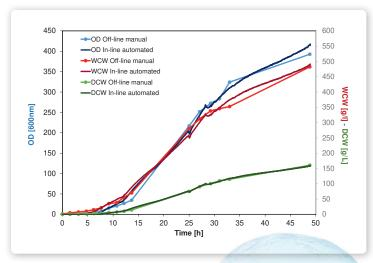
Figure 2: In-line turbidity versus off-line cell density measurements. The darker lines without dots represent the Dencytee in-line automated measurements. The lighter lines with dots represent TCD measurements from manual off-line reference methods.
